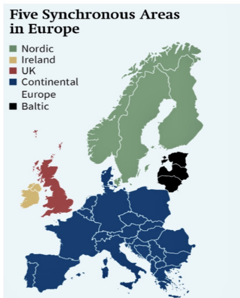
Map illustrating the synchronization of European Grids. The Baltics are to be synchronized in 2025. Source: Stiftung Wissenschaft und Politik
